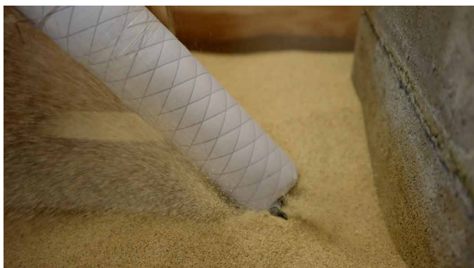
Movie 1. Overview of robotic burrowing with tip extension and granular fluidization. This video summarizes how tip extension, air fluidization, and asymmetry were used to create a soft burrowing robot.
